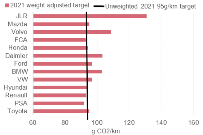
Figure 4: CO 2 fleet emissions targets vary across OEMs, adjusted according to typical weight of vehicles sold
